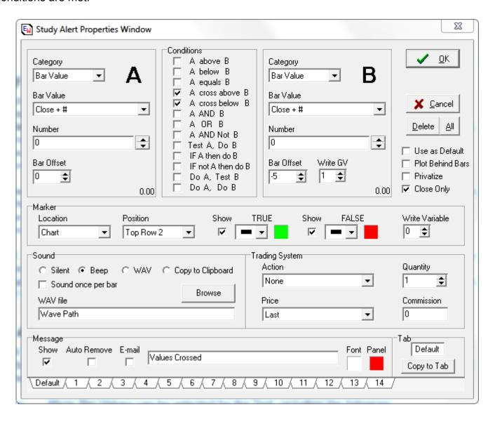
Panel 'A' and Panel 'B' are used to specify what chart or study values should be tested (to see if an Alert condition exists). The 'Conditions' panel specifies the relationship between the 'A' value and the 'B' value. For example, if the Study Value in Panel 'A' is greater than the Study Value specified in Panel 'B' then a Study Alert will be triggered and the appropriate action or Trade will take place.
