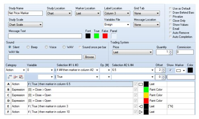
A – Display the Rectangle marker vertically at the Last price position and filled with the Black color. The marker's horizontal location is column 6.5, which is 52 pixels to the right of the last bar's plot position. Each column is 8 pixels in width.
